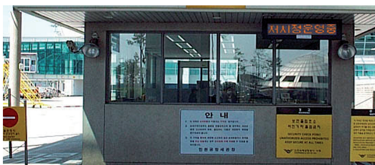
LVPs may include a warning system that is used to reflect the airport's status. In this case, a luminous panel on the building provides the necessary information. Incheon International Airport
