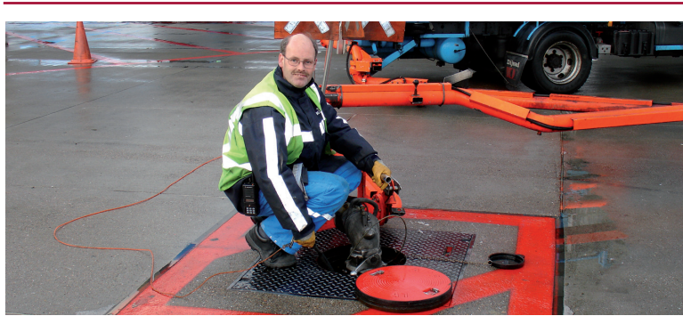
Electrostatic charges can be dissipated by grounding the fuelling vehicle and the aircraft. Amsterdam International Airport
